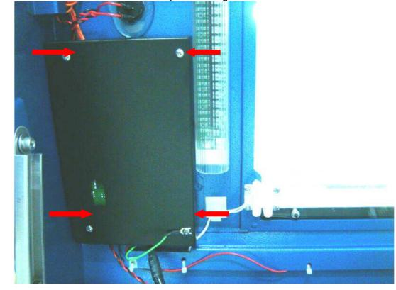
4. Dismount 4 screws for cover of control panel and ground cable screw.
