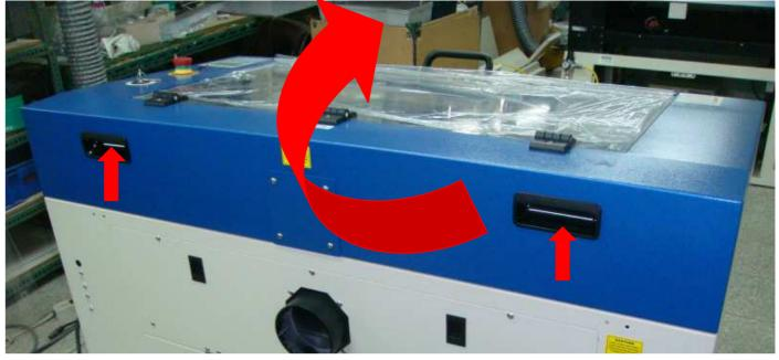
3. Please turn the safety lock switch to LOCK status according to the direction shown on the sticker (see picture) to avoid the collapsing of top cover.
